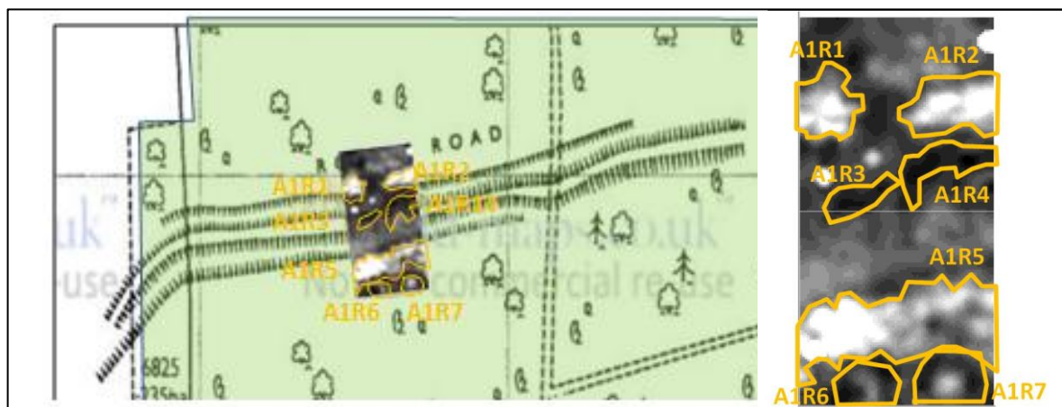
Figure 6.2 The Area A1 earth resistance anomalies
