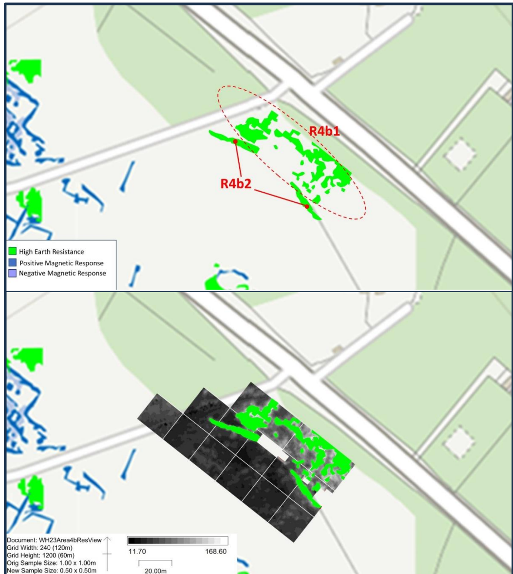
Figure 5.25 Earth resistance anomalies for Area 4b (Open Map, 2024).
