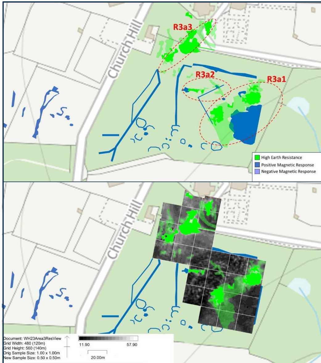
Figure 5.17 Earth resistance anomalies for Area 3 relative to the gradiometer anomalies (Open Map, 2024).
