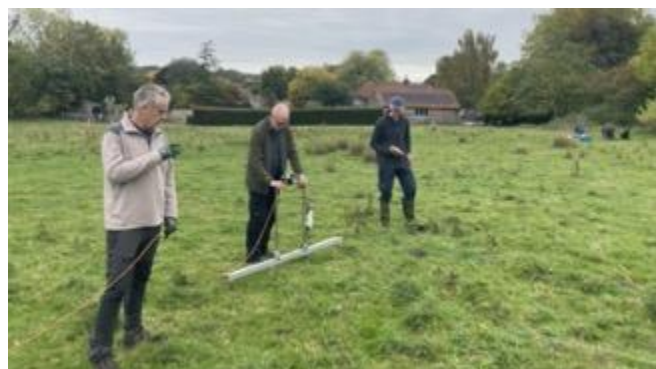
Figure 2: Tony, Eric and Philip collecting 0.5m resolution earth resistance geophysics data.
